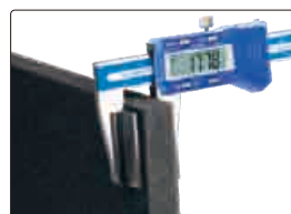
Measure thickness of rubber
