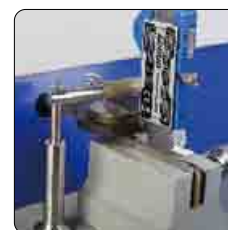
lapping measuring surfaces of caliper lower jaws
